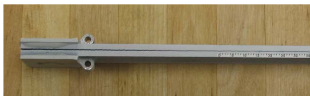
Figure 3 Tested laminate DCB specimen. [Color figure can be viewed in the online issue, which is available at www.wileyonlinelibrary.com .]
